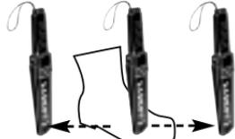
Interference Elimination Button may be required if floor rebar is present.
