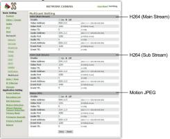
This function allows multiple people to watch video streaming without limited in the number of users, but is only applicable to the LAN environment. Video streaming format (H.264) is depended on the selected image format setting in Basic Setting — Video/Image — Video Format.
