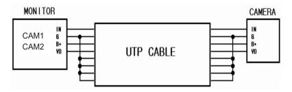
• If you use UTP CABLE[CAT.5], connect the rest 4 lines to GND after connecting 4 lines between monitor and camera.
